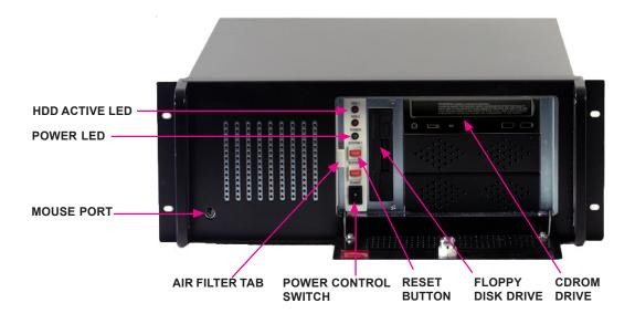
To access the front panel components, unlock and open the panel door. Located on the front of the Rack Computer are the following components.
